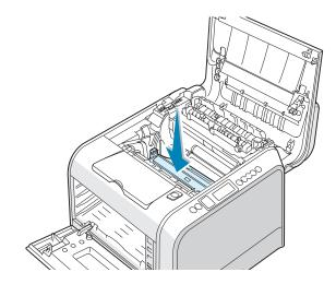
**CAUTION**: Replace the imaging unit carefully so as not to scratch and damage the surface of the green roller on the imaging unit.
